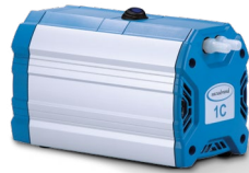
ME 1C Chemistry diaphragm pump 0.7 m 3 /h, 100 mbar Vacuum connection: Hose nozzle DN 8-10 (cannot be unscrewed)
