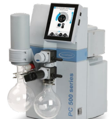
PC 510 select Chemistry diaphragm pump 2.0 m 3 /h, 7 mbar Vacuum connection: Hose nozzle DN 8-10
