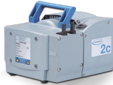
ME 2C NT Chemistry diaphragm pump 2.1 m 3 /h, 70 mbar Vacuum connection: Hose nozzle DN 8-10 (cannot be unscrewed)
