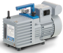
RZ 2.5 Rotary vane pump 2.3 m 3 /h, 2 x 10 -3 mbar Vacuum connection: Small flange DN 16
